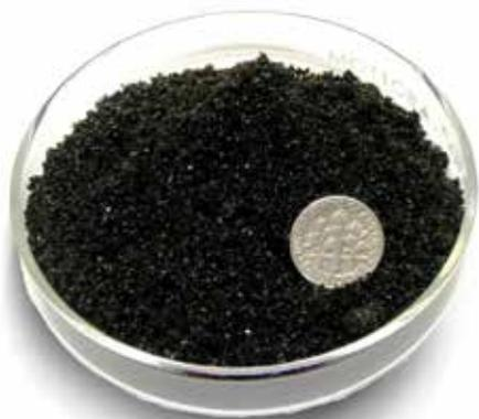
Free-flowing granules, primarily containing iron oxide, silica, alumina and calcium oxide.
