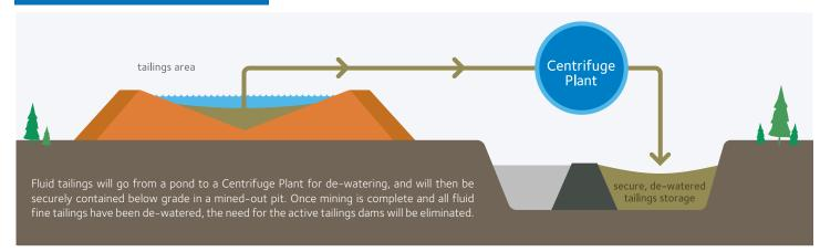
Tailings are a by-product of the process used to extract bitumen from mined oil sands. Tailings consist of water, silt, sand, clay and residual bitumen
