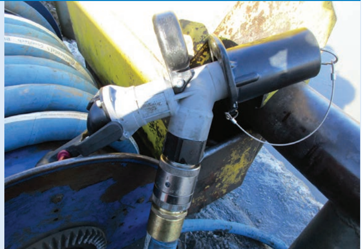
Fuel island hose with new swivel and break-away fitting. Thanks Jason and Robert!
