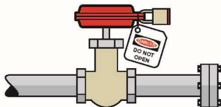
Figure 1: Open end of pipe with a blind. Nearest valve closed locked and tagged.
