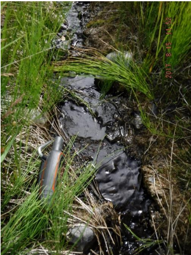
Photo I-34 Finger drain with geotextile – flow was estimated 0.5 L/min (PTD-2017-26)
