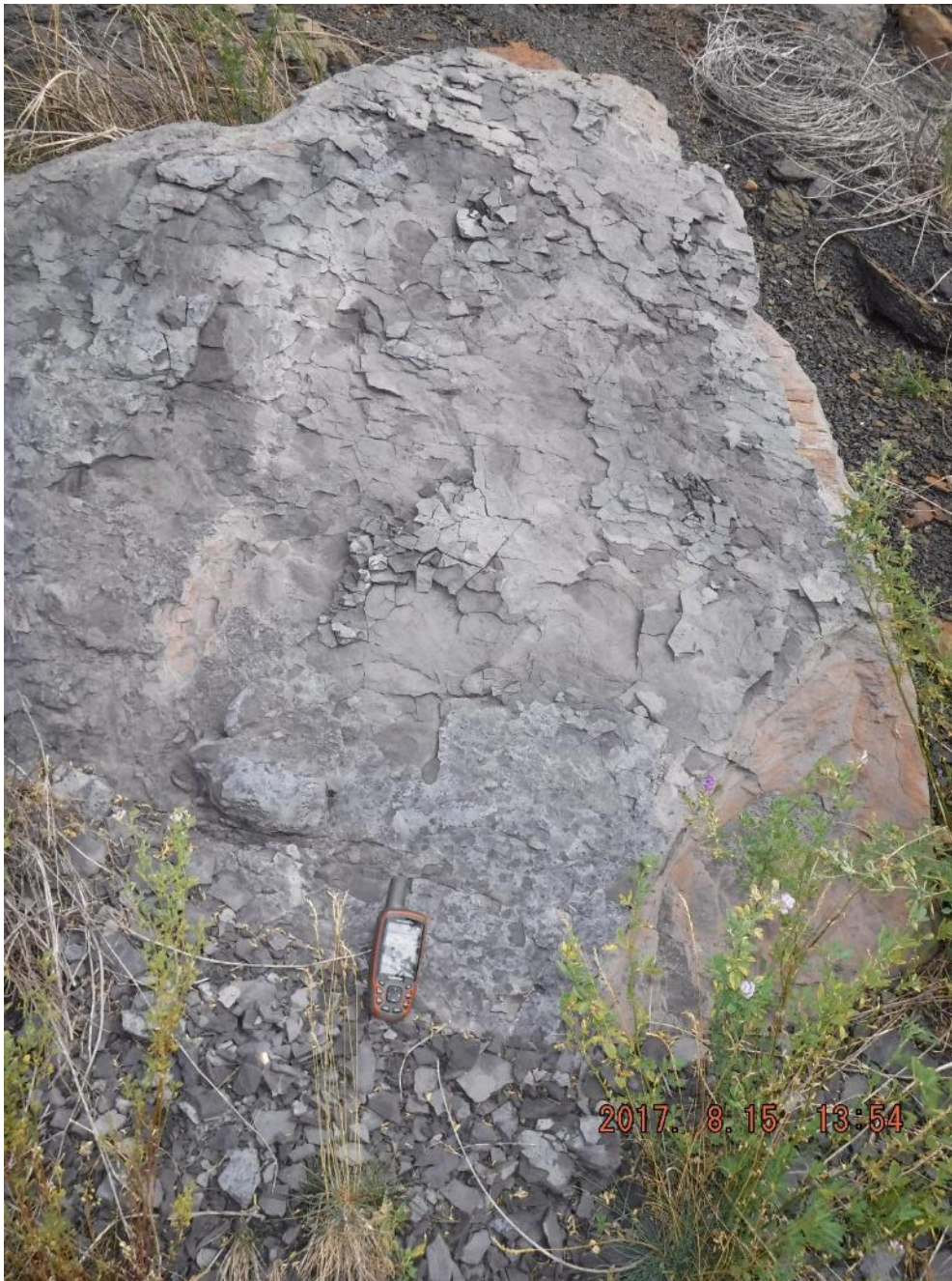
Photo I-54 Closeup of the slaking riprap (PTD-2017-43)
