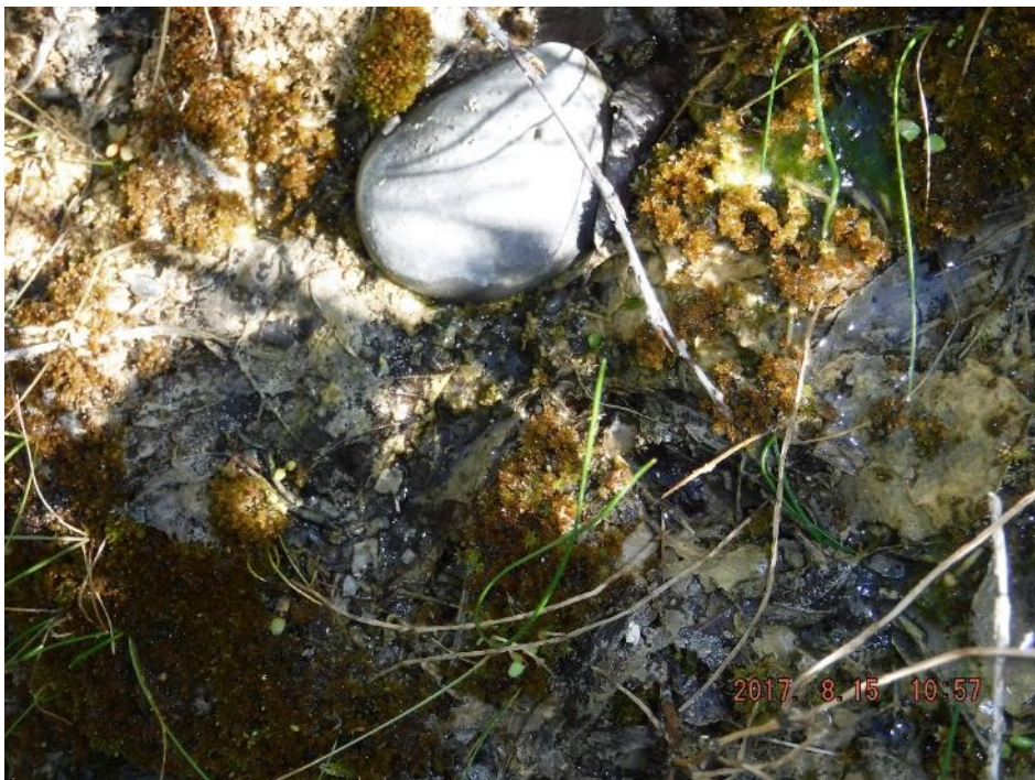
Photo I-27 Closeup of small flow (<1 L/min) downstream of the finger drain outlet (PTD-2017-21)
