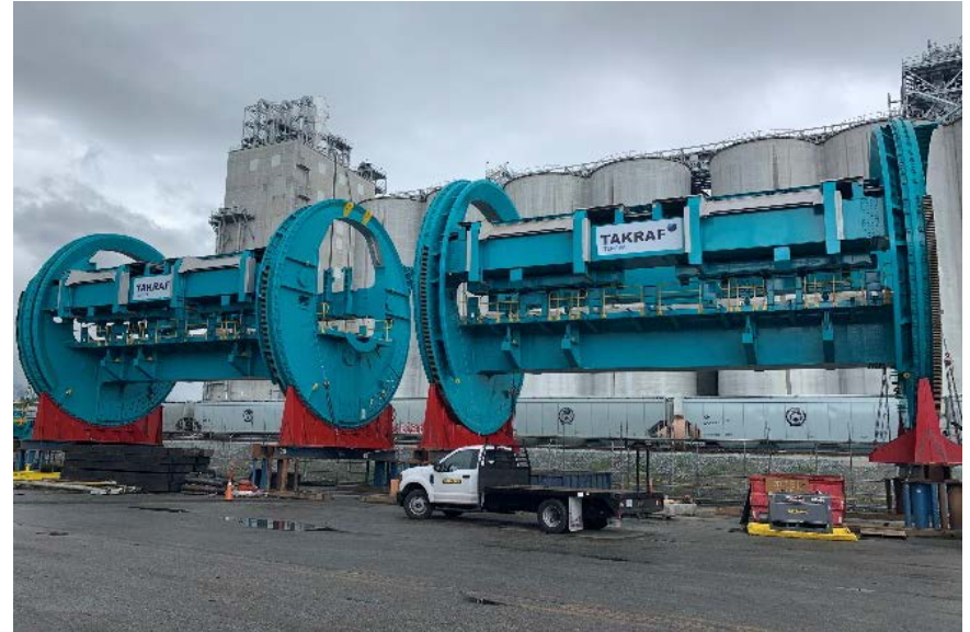
The new double dumper barrels, staged at Neptune in July 2020.
