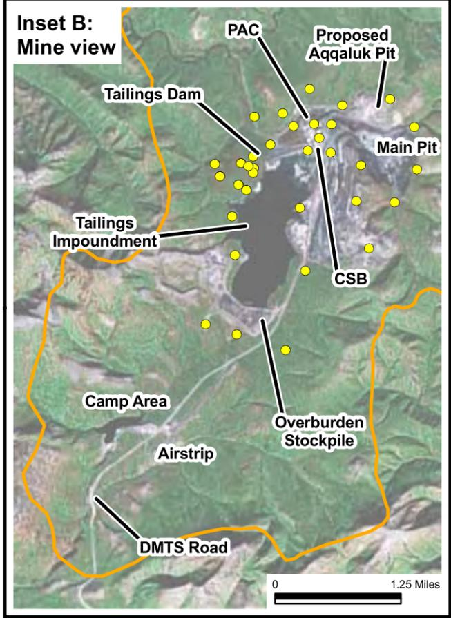
Figure 7. Dustfall jar monitoring stations
