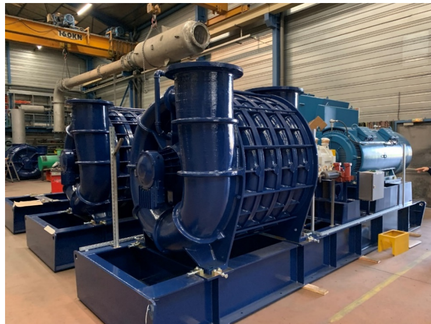
Final fabrication of flotation blowers in France. February 2018.
