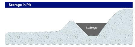
Tailings could also be stored in a pit after mining is complete. Slurry, thickened and dry tailings could be stored in this way. No additional footprint would be required, but use of the pit might reduce space available for other purposes such as water treatment or storage of waste rock.
