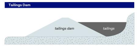
Slurry and thickened tailings can be stored behind a tailings dam. These structures are often used in the mining industry and the risks are well understood. Tailings dams need an appropriate area outside the pit(s) to store tailings.
