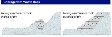
Slurry, thickened and dry tailings could be stored along with waste rock, either inside or outside of the pit. Neither option would require additional footprint, but storage outside the pit would may require additional efforts for water collection and management.
