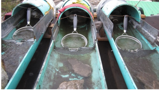
Figure 4.12 Strainers at the bottom of each stream
