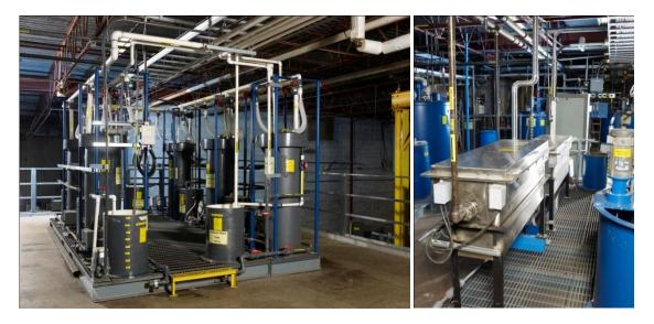
Figure 5 - CESL Gold Demonstration Plant ADR Circuit (CIC and EW Cells)
