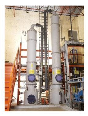
Figure 6 - CESL Gold Demonstration Plant Cyanide Recovery Stripper and Absorber Columns
