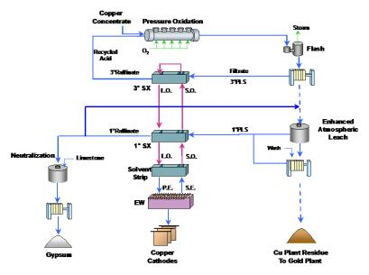
Figure 1 - CESL Copper Process Flowsheet
