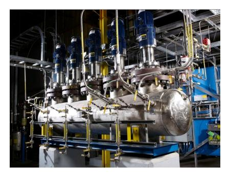
Figure 4 - CESL Gold Demonstration Plant Pressure Cyanidation Vessel
