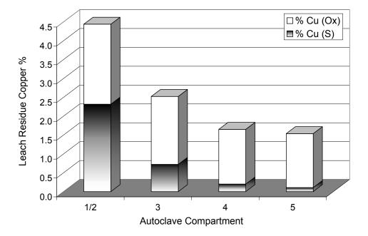
Figure 3 – Autoclave Extraction Profile at 60-minute Retention Time
