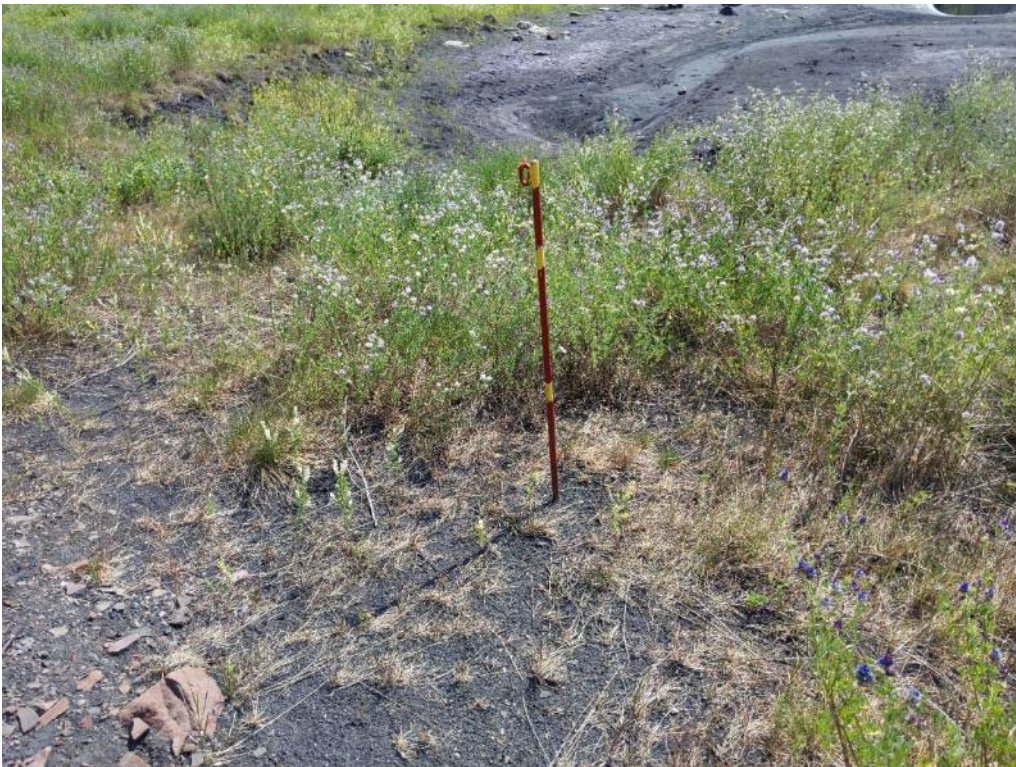
Photo I-11 Freeboard monitoring stake (SNTD-2021-09)
