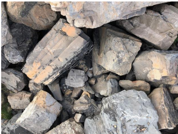
Photo 14: Weathering riprap at the emergency riprap stockpile
