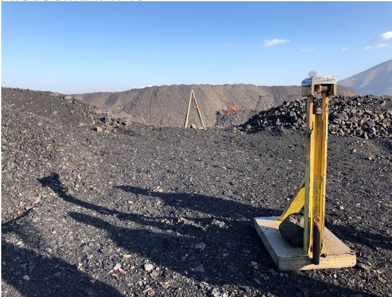
Edge of Eagle 4 South Backfill spoil - west side of active platform with extensometer, looking southeast
