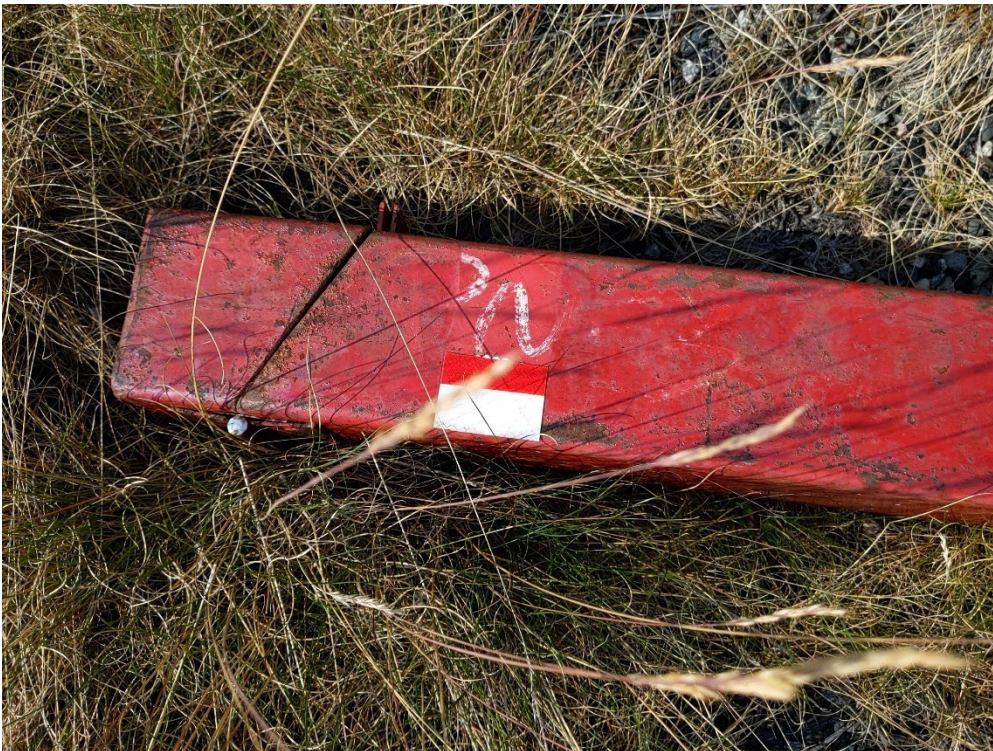
Photo II-27 Piezometer PN-3 needs repair (BTD-2021-16)
