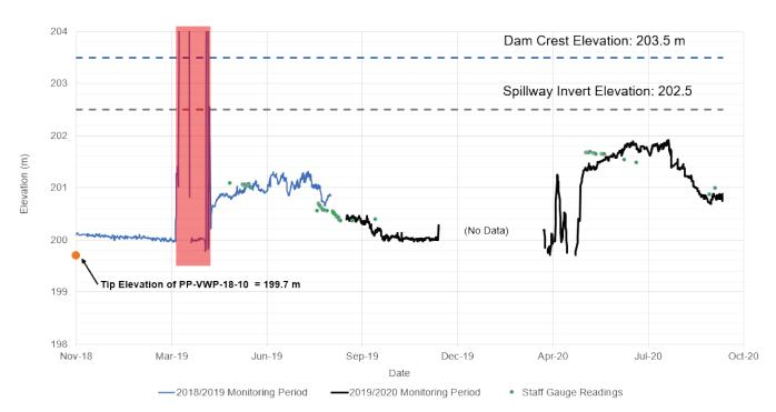
Note: Readings corrected for barometric pressure. Red shading indicates errors attributed to freeze/thaw. Data in green from staff gauge readings.
