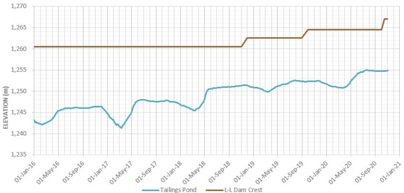
Figure 5.1 Highland TSF Pond and Crest Elevations: 2016 to 2020
