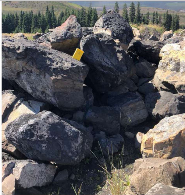
Photo 14: Weathering riprap at the emergency riprap stockpile.
