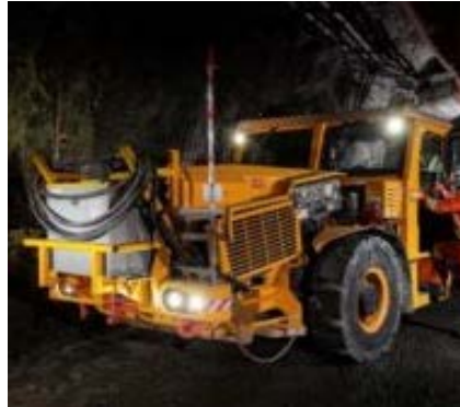
Electric boom vehicles to be tested in pit.
