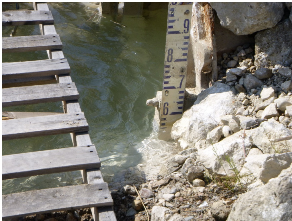
Photograph 19: Main Pond Water Level Gauge at Culvert Intake to Polishing Pond (Elevation 200.558 m), 12 August 2019
