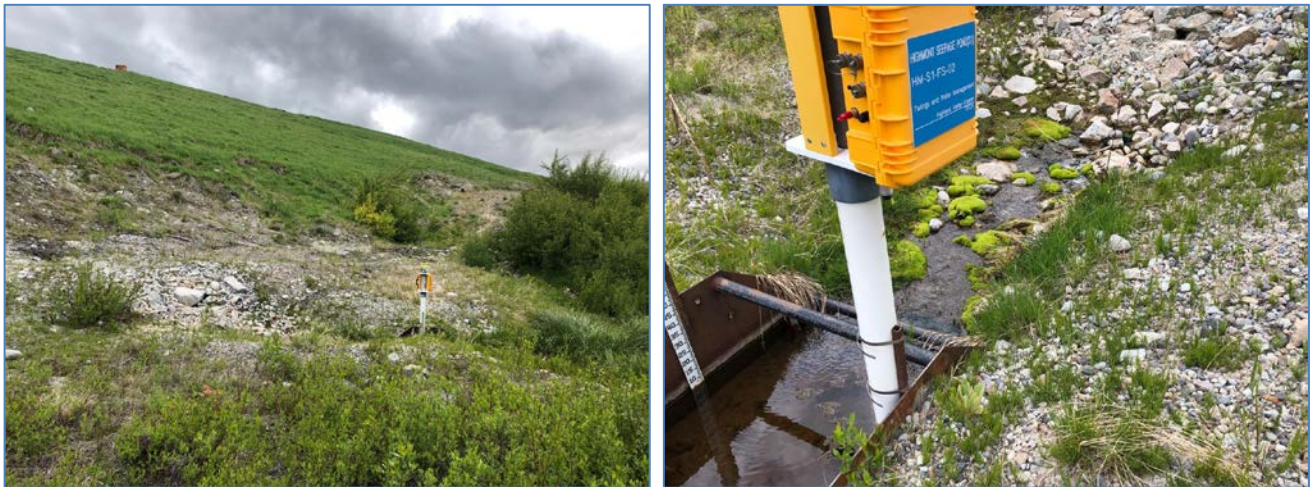
Photo II-A-12 Seepage flow measurement weir at toe of Highmont Dam (HM-S1-FS-02). Water flowing. (HGH-2019-12 and HGH-2019-13)
