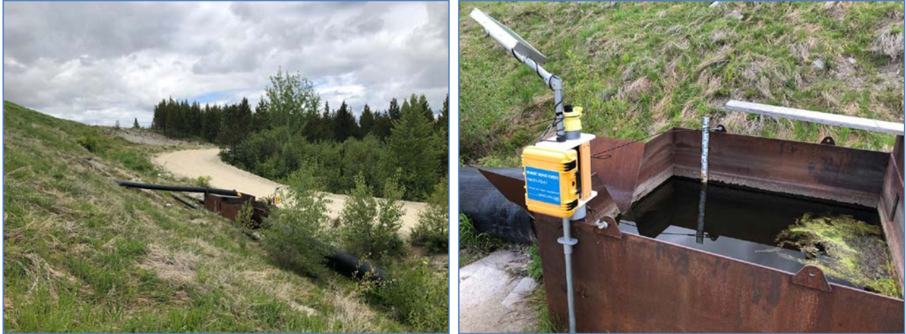
Photo II-A-12 Seepage flow measurement weir at toe of Highmont Dam (HM-S1-FS-02). Water flowing. (HGH-2019-12 and HGH-2019-13)
