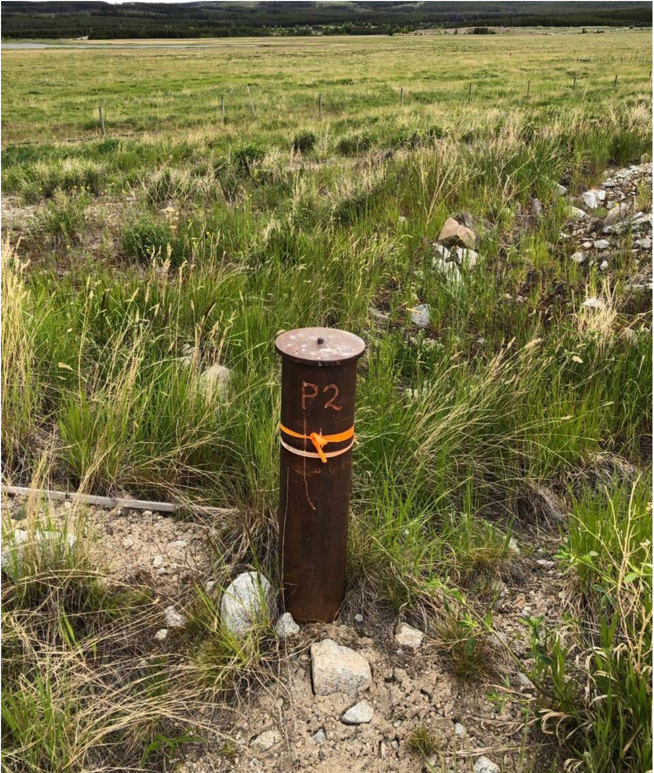
Photo II-A-3 Low spot on crest visible around P2 also demonstrated by contours on the plan view. No signs of distress, settlement or depressions. (HGH-2019-01)
