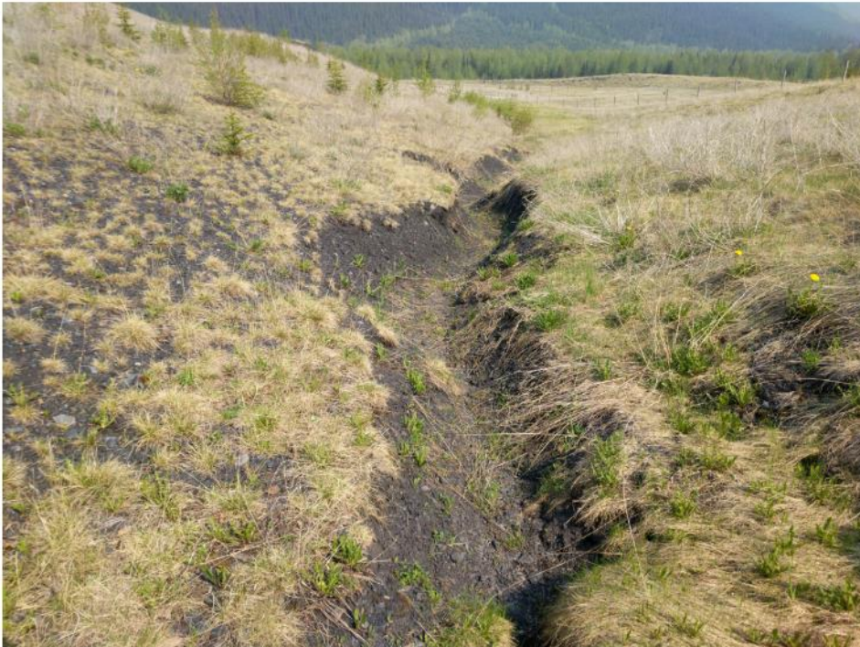
Photo II-15 BTD Toe. Erosion gulley observed during previous inspections. No obvious signs of change – looking north (BTD-2019-11)
