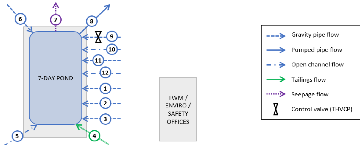
Figure 4.1 Flow Schematic for 7-Day Pond
