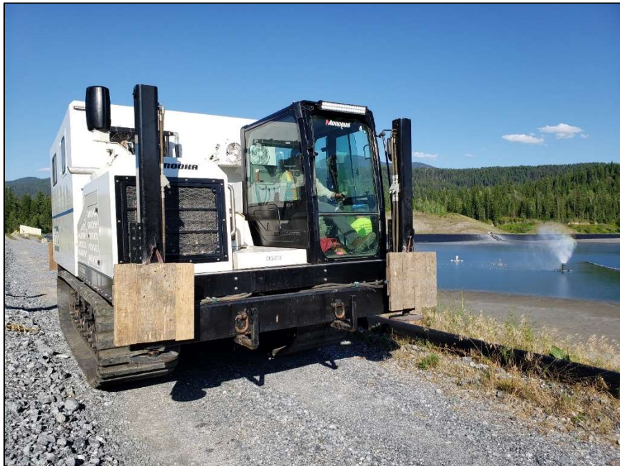
PHOTO 28 – Conetec CPT rig – Performing CPT on crest of dam.
