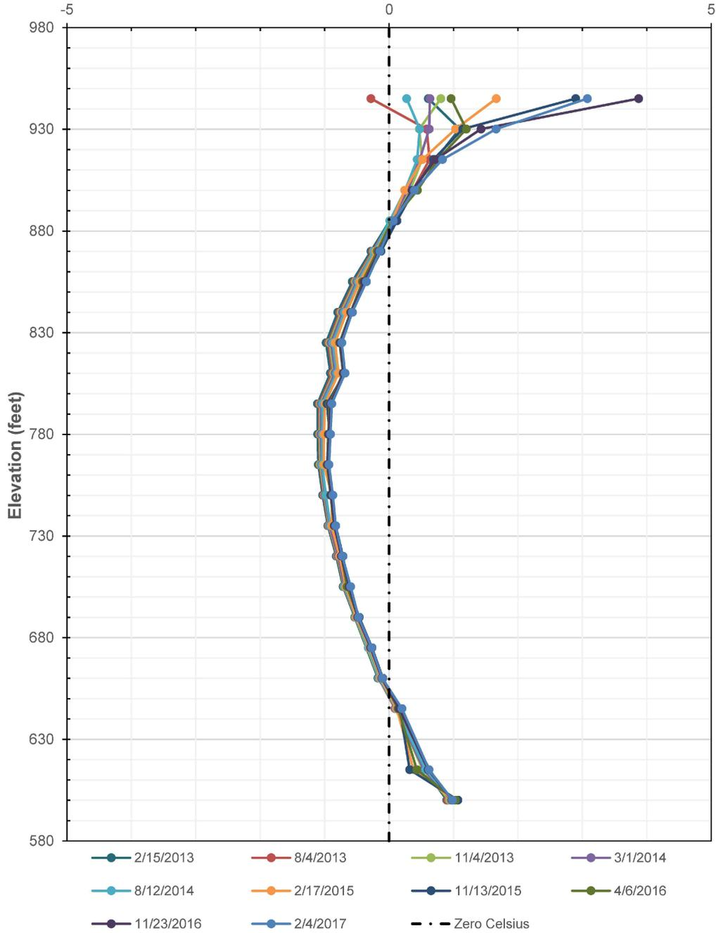
Last Edited By: bhiles Date: 2018-10-24 Time: 4:02:07 PM | Printed By: SANDERSON Date: 2018-11-05 Time: 12:52:56 PM Path: \\anchorage\Public\Geomatics\Tech\Reef\DogR... PROJECTS\1895982 TAK 2018 RD Main Dam Annual Inspection\Task 2000 TMD\02\_PRODUCTION\DWG... | File Name: Appendix C Raw Thermistor Data.dwg
