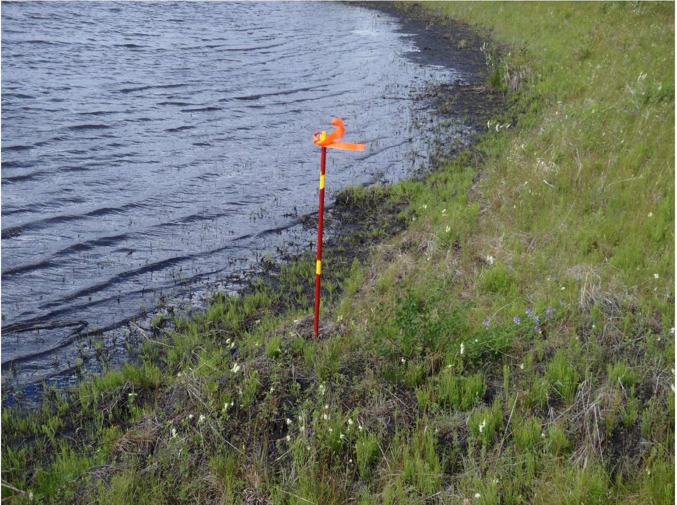
Photo I-52 Permanent Poned Area 1 extent marker installed by Teck in July 2018 for pond level monitoring (near PTD-2018-25)
