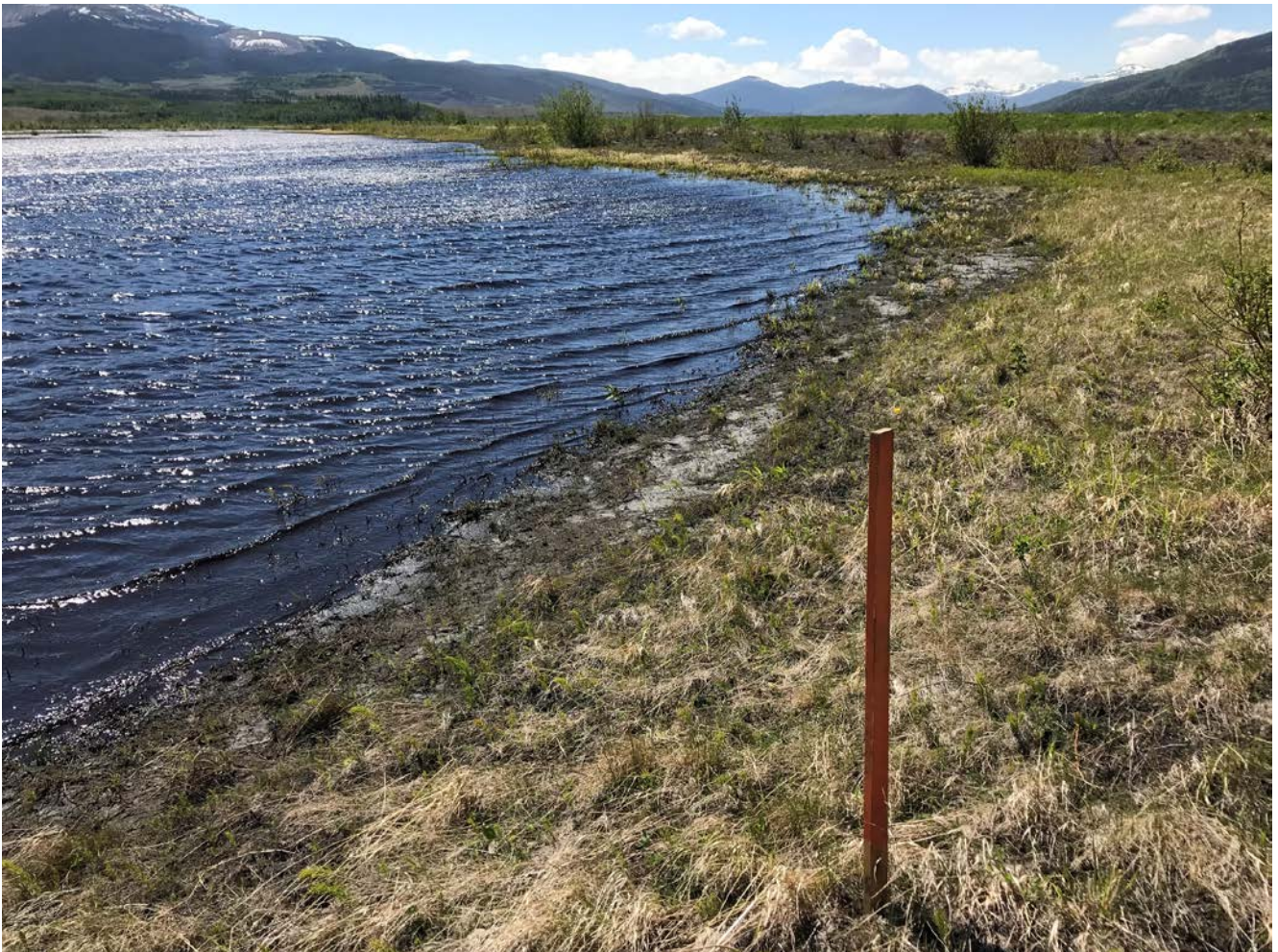
Photo I-36 Temporary stake installed at the ponded area at the northwest corner of the PTD for freeboard monitoring. A permanent staff gauge was installed in July 2018 (PTD-2018-25)
