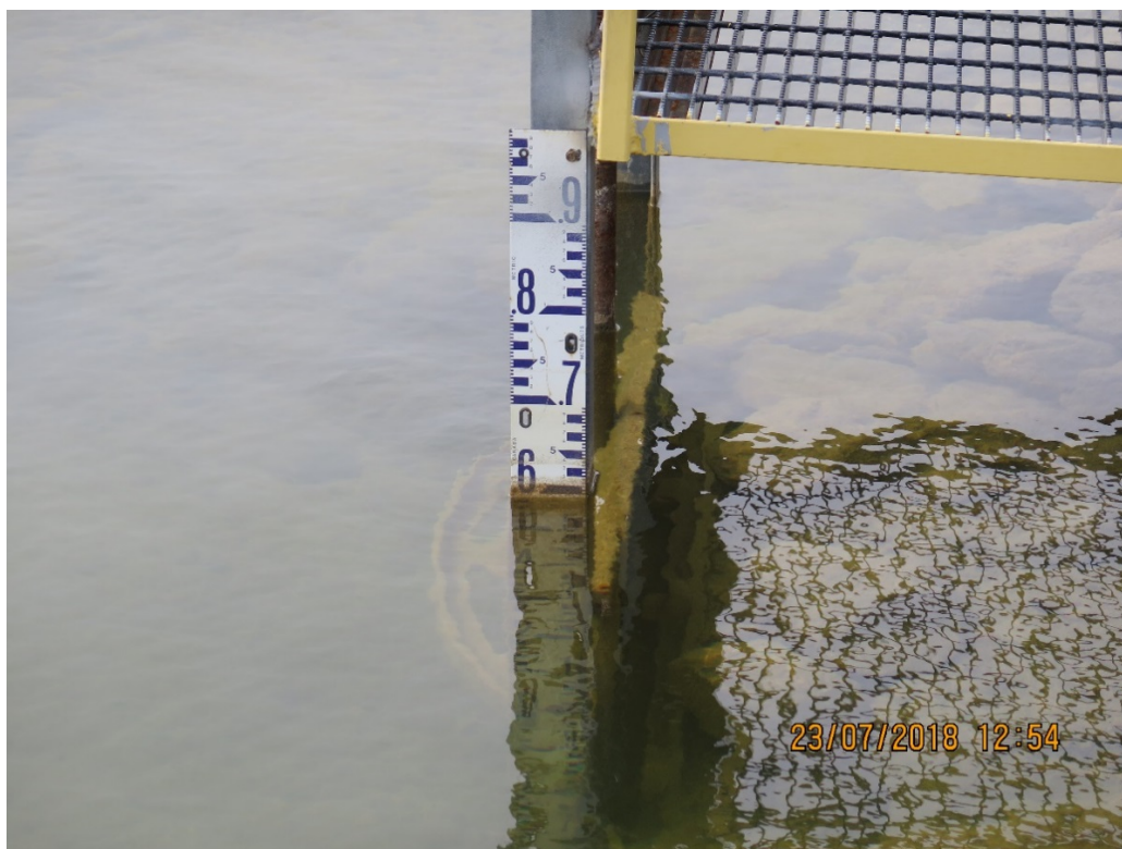
Photograph 17: Main Pond Water Level at Culvert Intake to Polishing Pond (201.62 m). 23 July 2018
