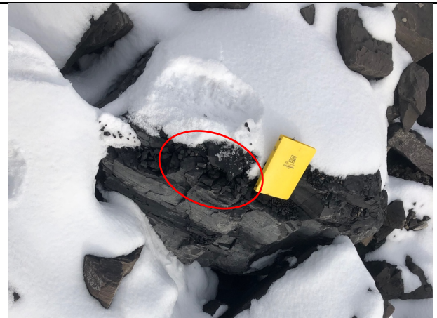
Photo 4: Riprap degradation due to weathering on a surface of a piece of riprap (red outline)
