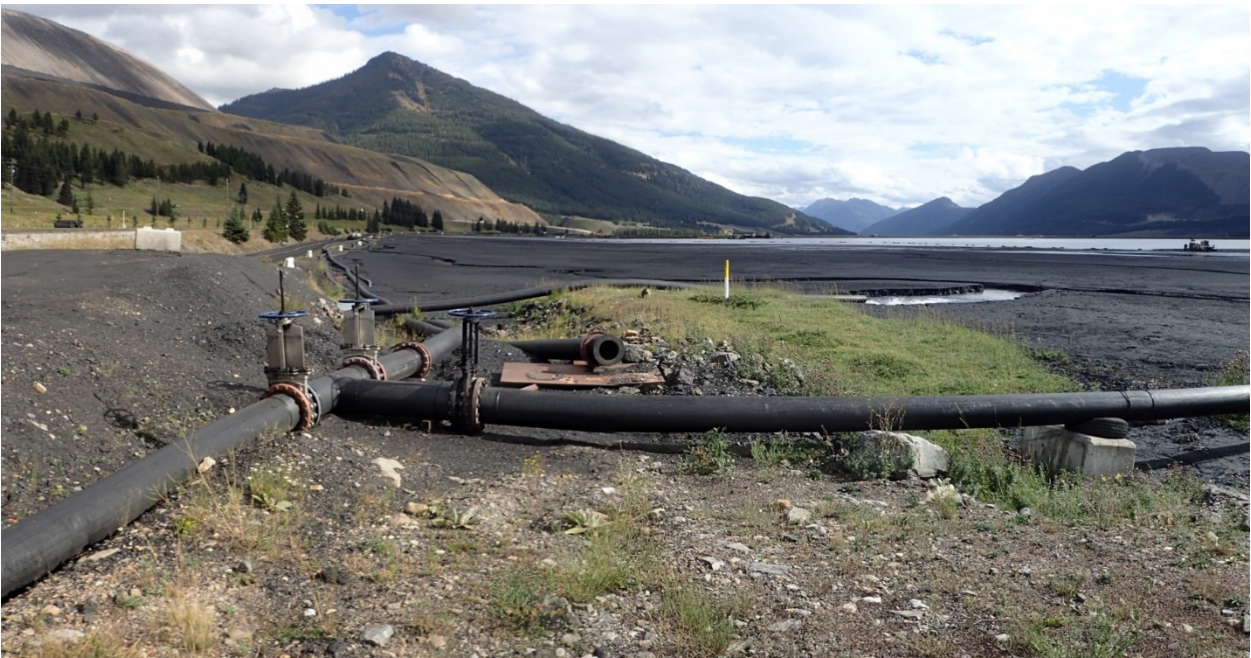
Photograph A-17: Tailings dredge pipeline and emergency bypass in foreground, temporary reclaim pipeline from Turnbull TSF discharging water along with Blackmore creek culverts, looking south, 11 September 2018.
