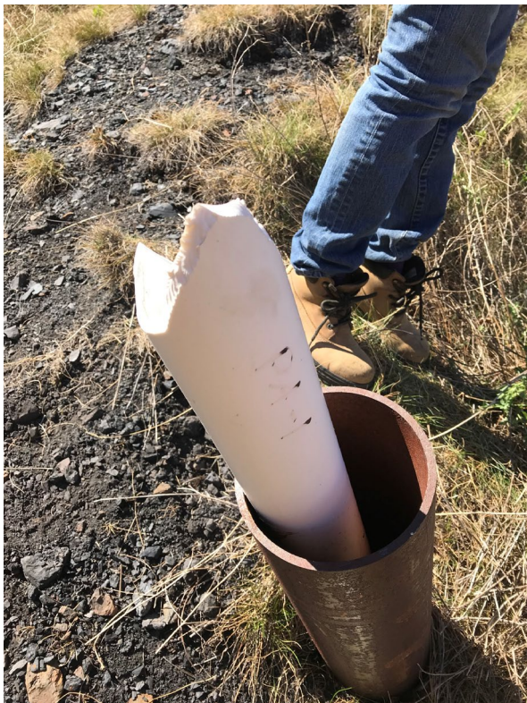
Photo II-7 Standpipe piezometer PA-1 – top of casing requires trimming (BTD-2018-04)
