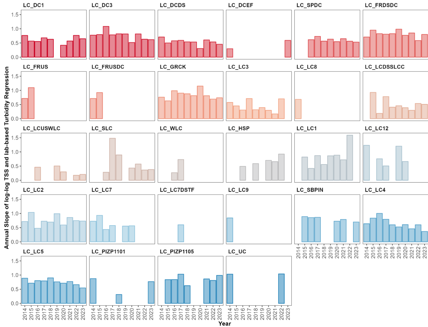
Figure A6 Annual slope from regression of log-transformed TSS against lab-based turbidity; data from specific years were excluded if <3 data points were collected in a year, or if the slope of the regression estimate was lower than or approaching zero. Data from years with y-intercept values less than zero were additionally excluded.
