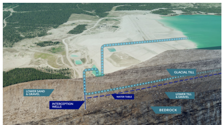
Through the Sulphate Adaptive Management Plan, interception wells were installed starting in 2017 to capture seepage and return it to the Highland Tailings Storage Facility.
