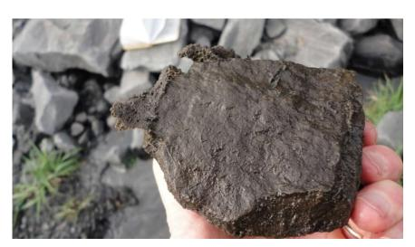
Figure 1. Partially Concreted Sample. Note calcite on the left side edge, which has extended beyond the substrate sample.
