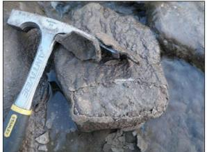
Calcite scale - a relatively thin, crystalline coating, which is homogenous in texture.
