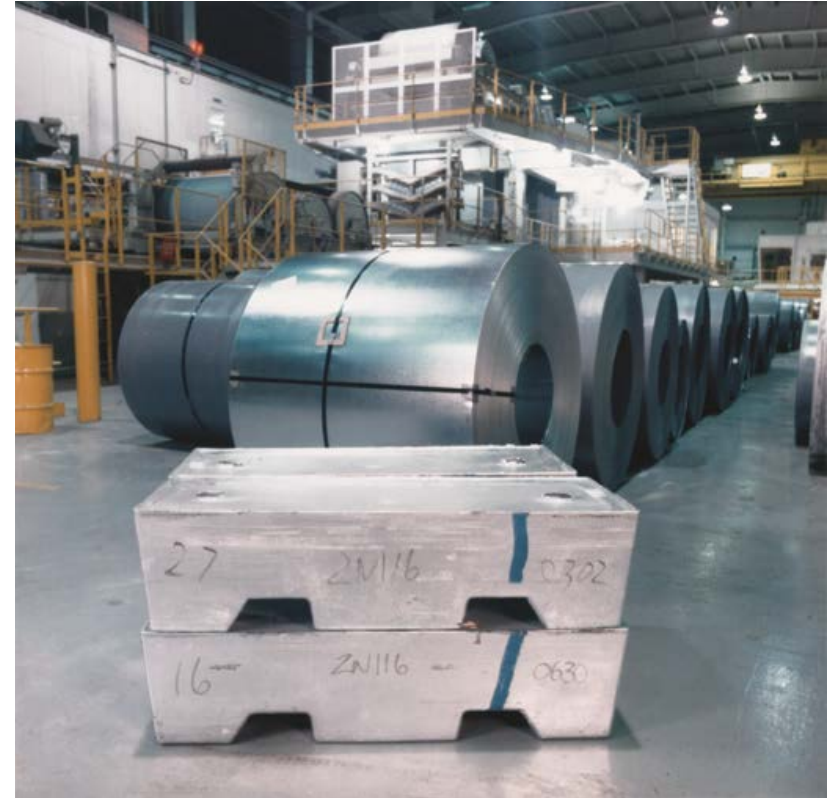
Tailor-made zinc jumbos with galvanized sheet steel
