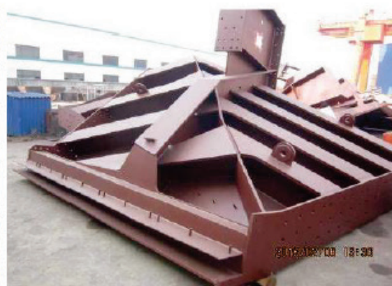
Hopper side walls had been checked after painting
