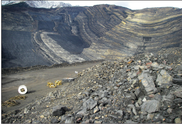
High pit wall at Line Creek Operations showing coal-bearing strata
