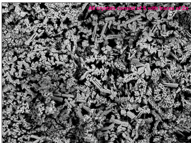
Scanning electron microscope photograph of elemental sulphur in test samples
