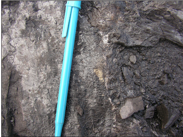
Pyrite in coal host rock
