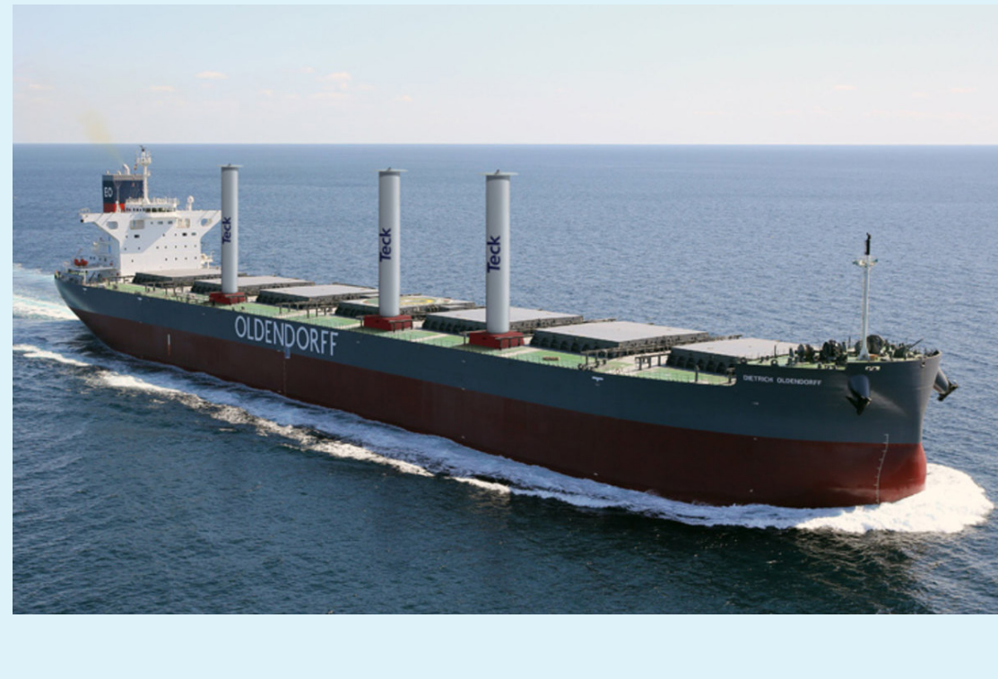
Pictured: A rendering of the Oldendorff ship outfitted with a Flettner Rotor system.
