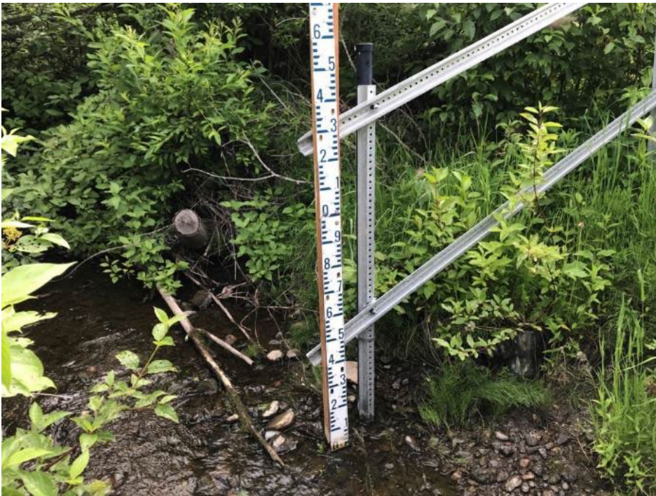
Photo II-46 Flow monitoring station immediately upstream of Pinchi Lake Road culverts
