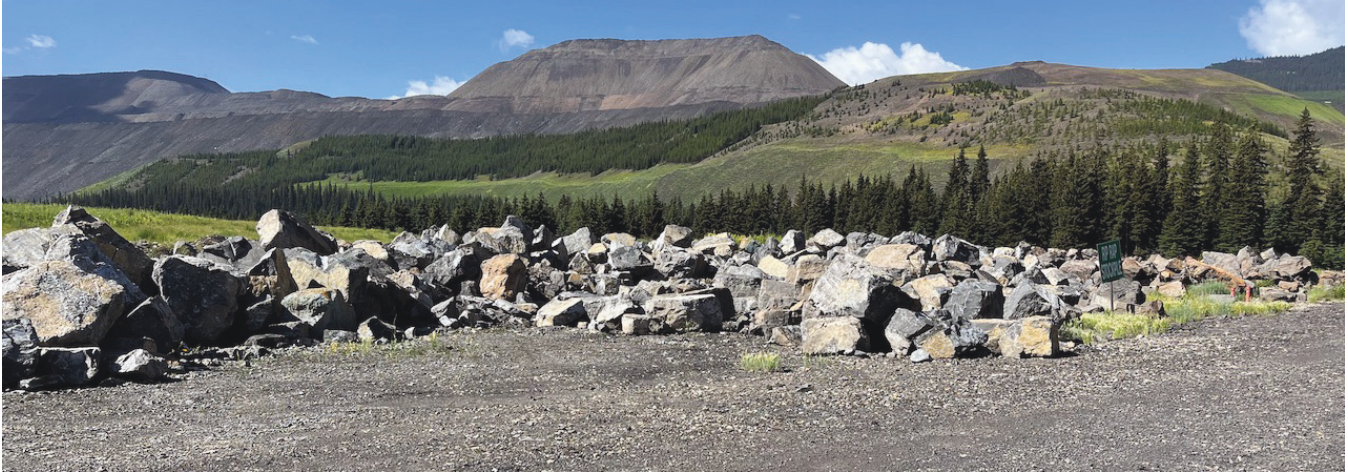
Photo 13: Emergency riprap stockpile south of STP
