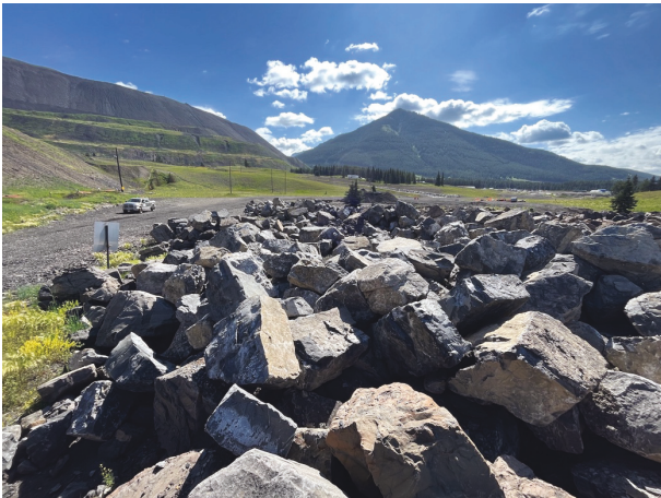
Photo 14: Riprap at emergency riprap stockpile
