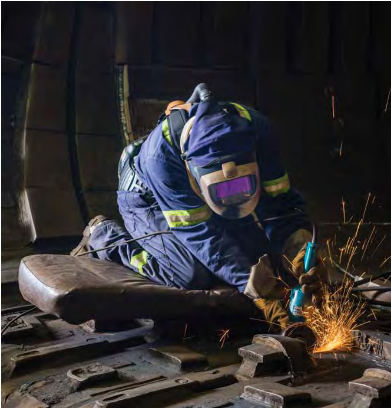
Pictured above: Welder Pete Kliment repairs a shovel bucket at Fording River Operations in B.C., Canada
